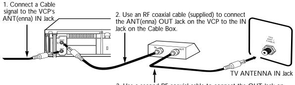
3. Use a second RF coaxial cable to connect the OUT Jack on the Cable Box to the ANTENNA IN Jack on the back of the TV.
